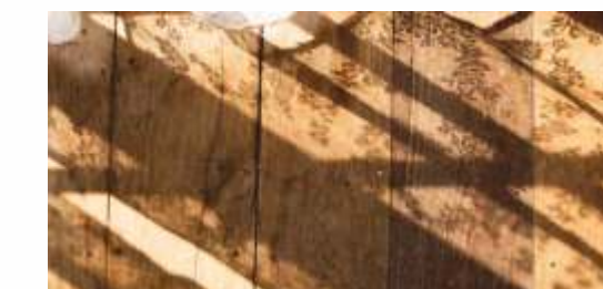
Avoid Direct sunlight / continuous light form the HPL Sheet These may cause to color fading due to UV Rays
