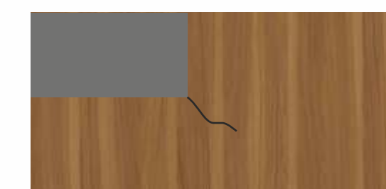
NO CLAIM WILL BE ENTERTAINED FOR CRACKING ARISING OUR OF ROOVE CURVING OR L. SHAPE
